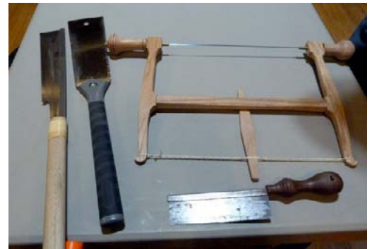
Various saws used for cutting dovetail joints
