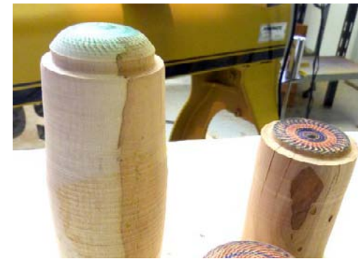
Examples of chatter patterns on end grain, colored with a sharpie
